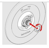
Remove the lower brass ring (temperature setting ring) and rotate the brass ring clockwise to increase temperature or anti-clockwise to decrease. Refit to spline in new position.
