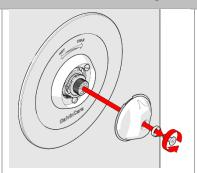
Unscrew the tamper proof screw from handle. Pull out handle assembly from the body.
