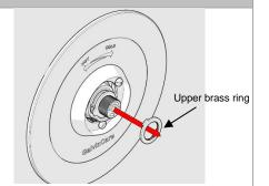
Remove the upper brass ring (closure setting ring). Make sure the control rod doesn't rotate during the next steps.
