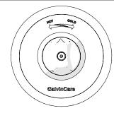
8. Ensure a plastic washer is located in a handle outer groove. Adjust the handle so the arrow shape on top of the handle matches the marking on the faceplate. Squeeze the plastic washer, push the handle into the flange, and fasten the screw.
