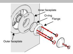
1. To isolate the shower, remove the handle and flange by unscrewing and carefully remove the inner faceplate and o-ring. (As shown)
