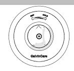
As the handle is rotated anti-clockwise the delivered water progresses from cold through warm to the pre-set maximum temperature of approximately 41°C.
